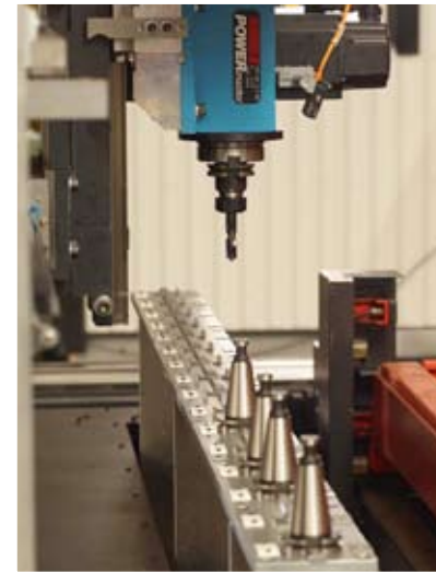
Tool machine, 16 positions
